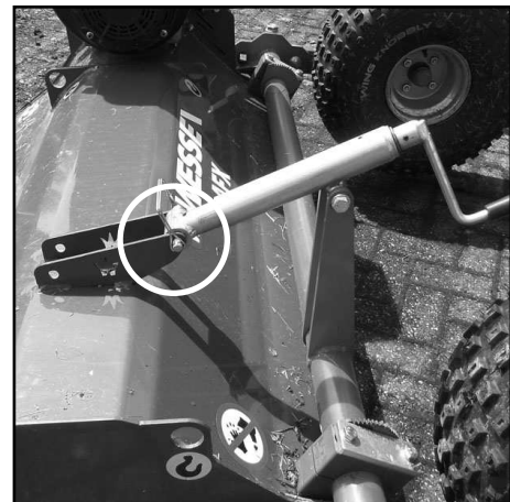
Adjuster position when wheels are set to the Rear of machine
